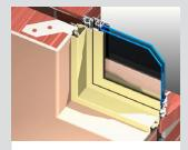
Custom building-in lugs secure the jamb to cavity brick wall.
